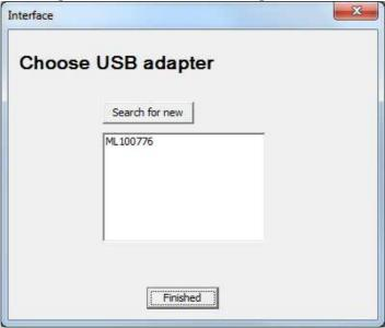
The serialnumber is written on the USB adapter. If none is appearing in the list the following must be checked:
